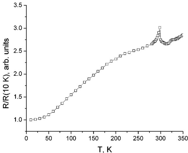
FIG. 4. Temperature dependence of resistance for  $\text{Ni}_{54}\text{Mn}_{21}\text{Ga}_{25}$  alloy.
