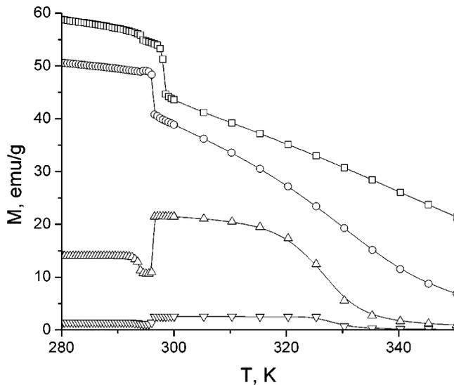
FIG. 3. Dependences of magnetization vs. temperature for  $\text{Ni}_{54}\text{Mn}_{21}\text{Ga}_{25}$  at different applied magnetic fields:  $H=100$  Oe ( $\nabla$ ),  $H=1000$  Oe ( $\Delta$ ),  $H=10000$  Oe ( $\circ$ ), and  $H=50000$  Oe ( $\square$ ).
