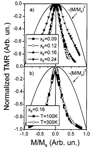
Fig. 2. Normalized TMR as a function of normalized magnetization for  $(Co_{50}Fe_{50})_x(Al_2O_3)_{1-x}$  cermet films of (a) different composition and (b) at different temperatures.
