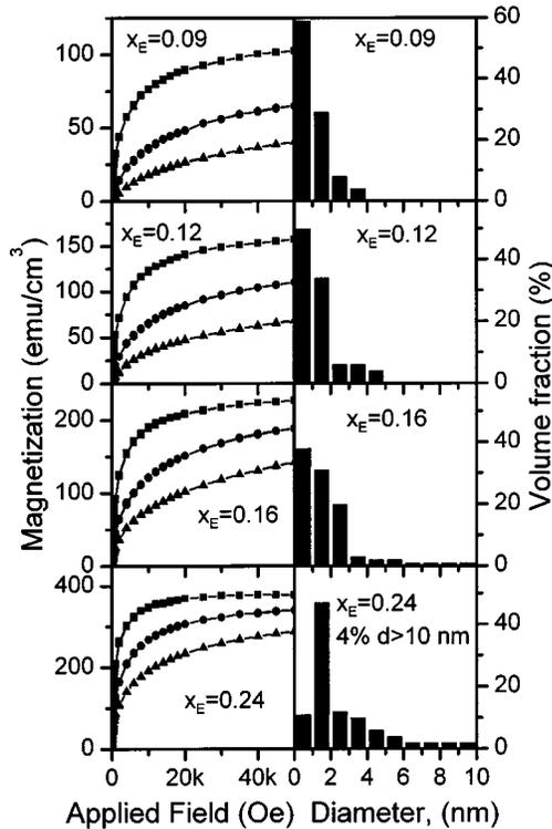
Fig. 1. Magnetization as a function of applied field at 10 K (■), 100 K (●) and 300 K (▲) (left side) and corresponding particle size distribution (right side) for  $(Co_{50}Fe_{50})_x(Al_2O_3)_{1-x}$  cermet films of different composition.
